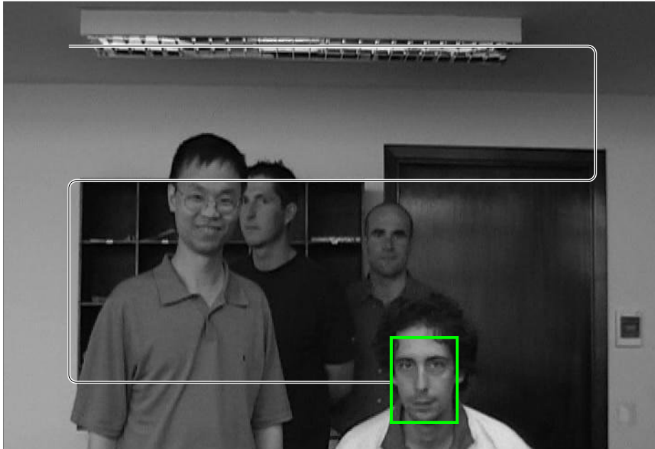
Fig. 1: In TLD, a binary ensemble classifier is used to locate the object of interest by applying it in a sliding-window manner. The ability for multi-scale detection is achieved by scaling the size of the detection window. Image is from the SPEVI 1 dataset.
